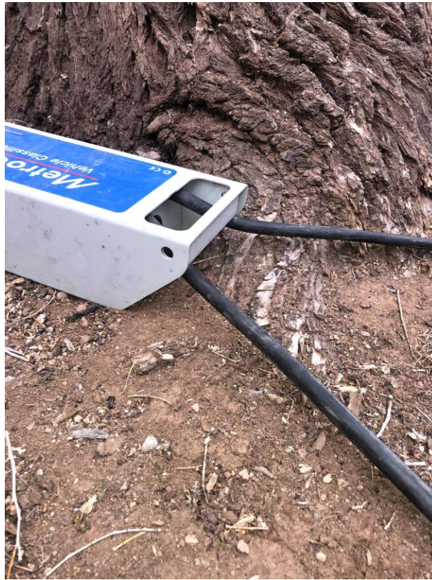
Figure 3: Vehicle counter used by RRC Associates to collect data relating to the ORV Indicators.
